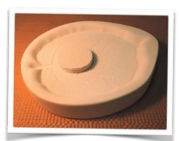
This plug is used to make a hole in the cast leaf. Note: If  $\frac{1}{8}$ " fiber paper is not available, use a combination of other thickness to get the same results.
